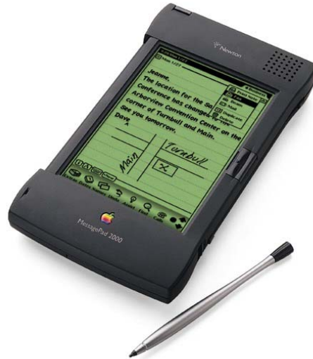
Figure 5. The Apple Newton was one of the first widely used PDAs. Dragon Systems created a voice recognition system for it.
