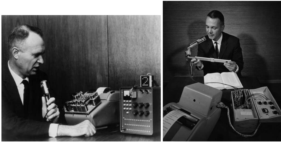
Figure 2. The IBM “Shoebox” (1962) could do simple addition and subtraction purely by voice command.
